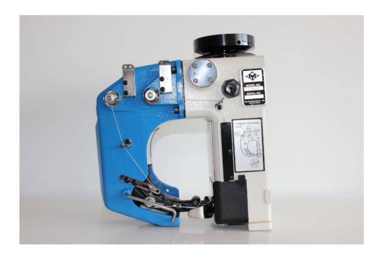
Stationary bag closing machine Yao Han F900A is a very popular model of industrial stitchers, designed for mounting on a tripod or column. Model F900A is a reliable single reinforced stitch (2-thread) designed for stitching different kinds of bags: paper, cotton, PP/PE, hessian, jute etc.
